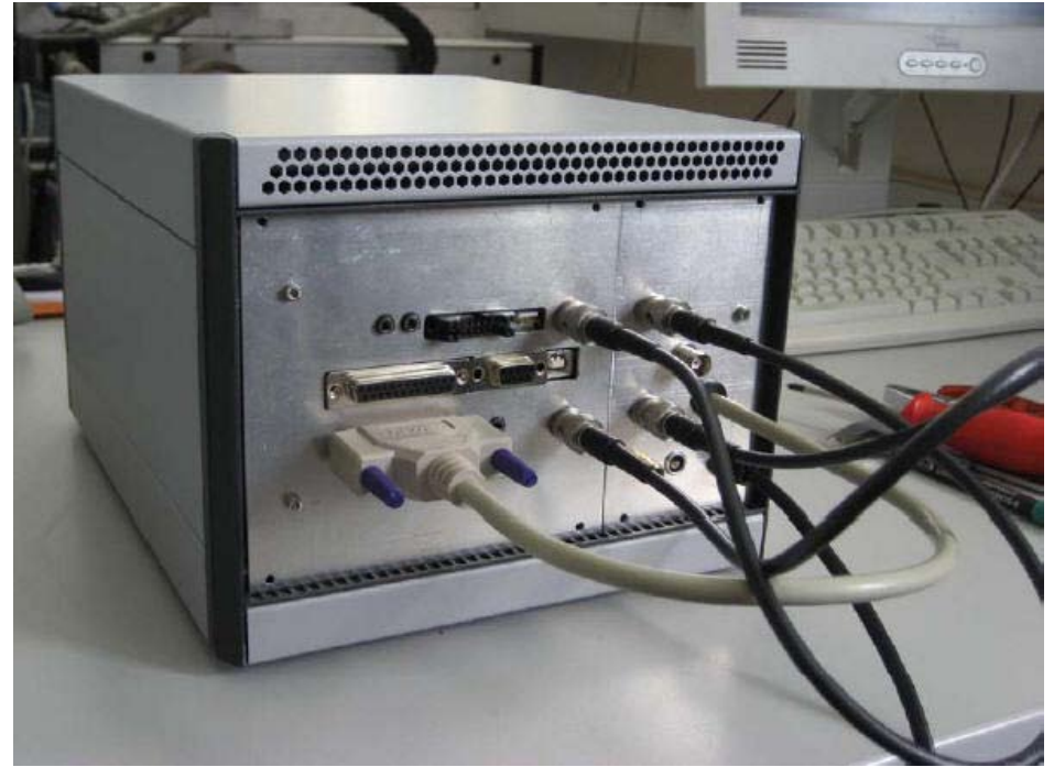
Fig.4: View to the closed unit. On the right side another board is mounted which connects Mercury and Penelope to the T/R relays' inside the box. This will later be replaced by the two Alex boards.
