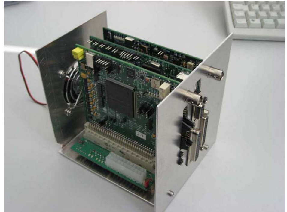
Fig.2: The connector side of the boards is closed with an aluminum sheet too. All notches have been worked out very carefully resulting in good fitting accuracy; the boards are therefore nicely fixed in the Atlas slots allowing for any mounting orientation.
