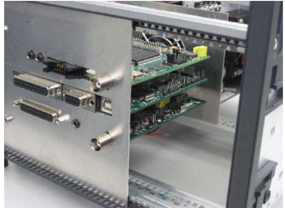
Fig.3: The assembly in the housing is then accomplished by turning 90 degrees and shifting into the red EU card tracks to the left. The empty space on the right side is foreseen for the Alexiariis boards.
