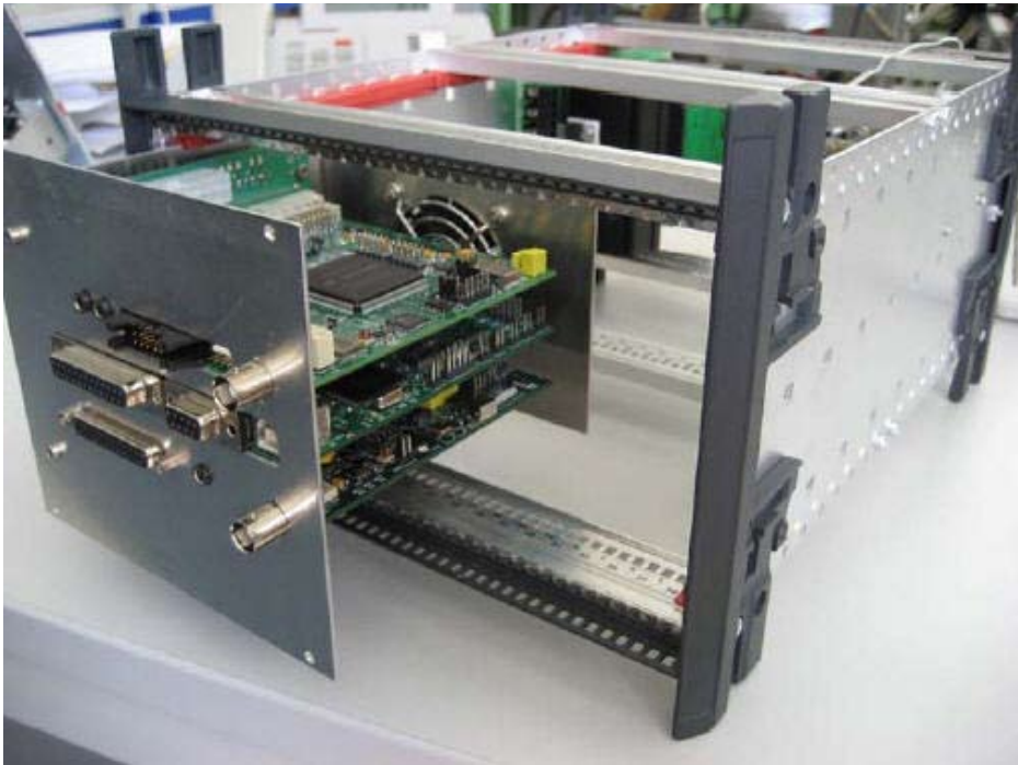
Fig.3: The assembly in the housing is then accomplished by turning 90 degrees and shifting into the red EU card tracks to the left. The empty space on the right side is foreseen for the Alexiariis boards.
