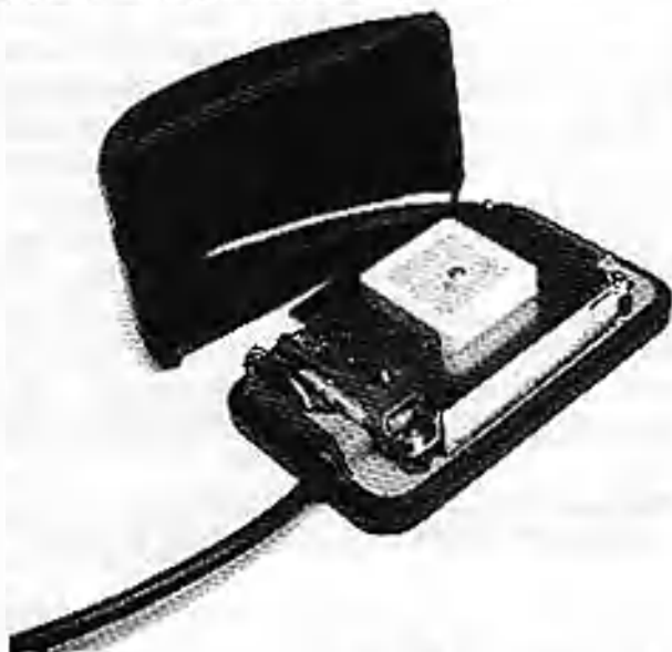
View from above and behind. Good view of patch antenna
