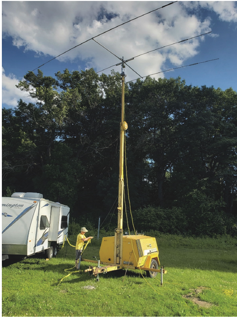
An Allmand Brothers ML4- larger and wider with a tri-band beam, dipoles and electric hoist.
