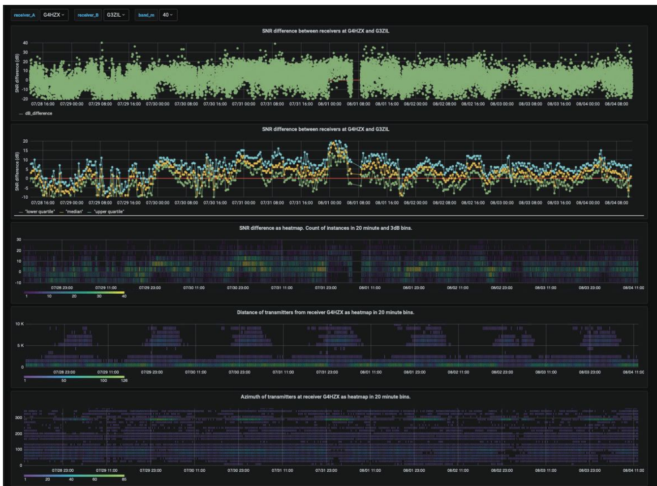
Figure 6. As postgresQL is a relational database that allows self-joins a query in Grafana can return data derived from one or more receivers. This Dashboard shows the SNR difference between G3ZIL and G4HZX on 40m, for spots from the same sender at the same time, as a time series scatter plot in the top panel, as median and lower and upper quartiles in the second panel and as a heatmap in the third. Heat maps of spot distance and azimuth at G3ZIL help interpret the SNR difference.
