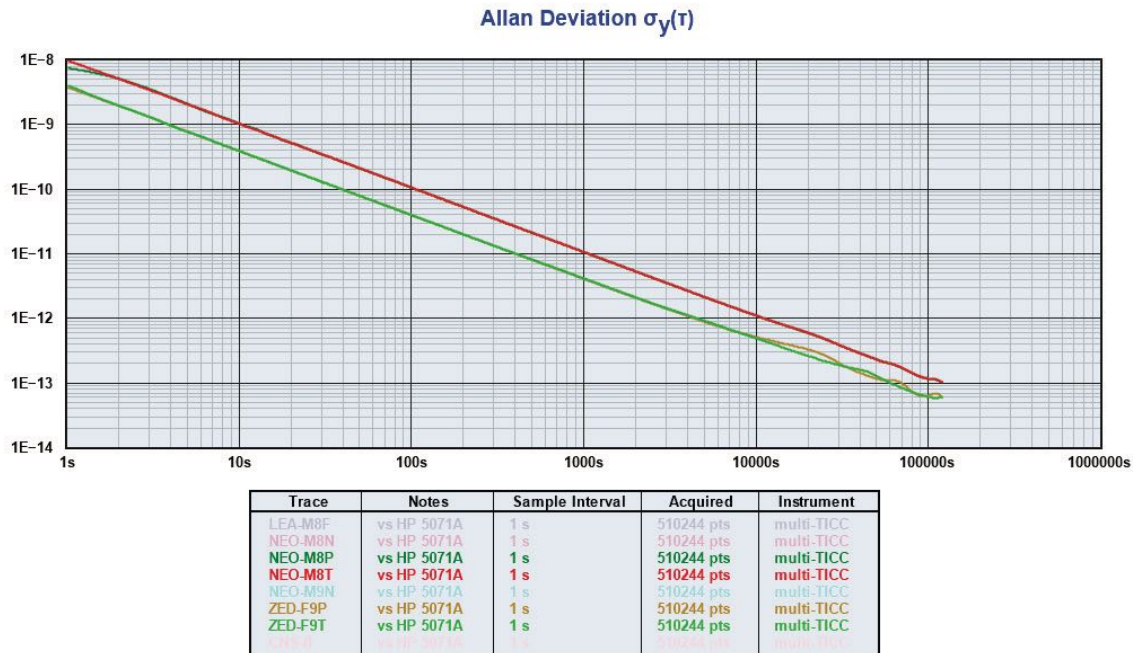
Figure 14: Positioning/Timing Receiver Allan Deviation Comparison
