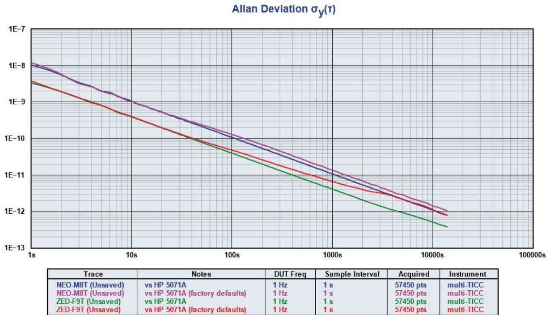
Figure 27: Allan Deviation of Timing vs. 3D Navigation Solution
