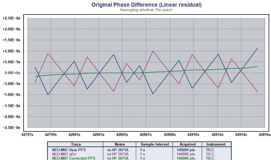
Figure 25: Quantization Error and Correction
