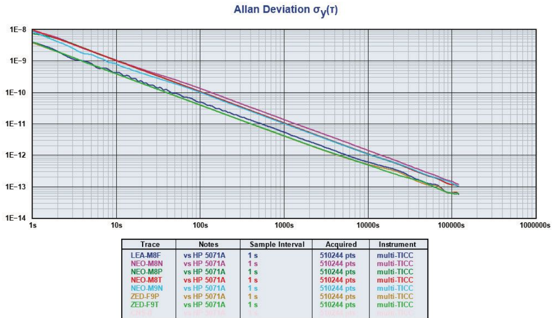
Figure 2: Allan Deviation of all seven u-blox receivers.
