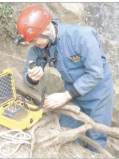
A HeyPhone in use on the surface above Carlswalk Caverns in Derbyshire.
