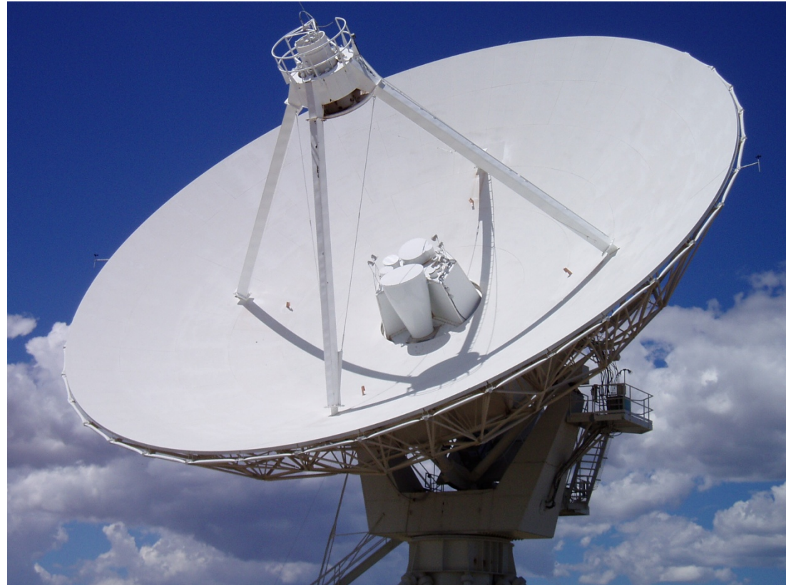
Antenna 24 – the first EVLA antenna outfitted with all eight feeds.
