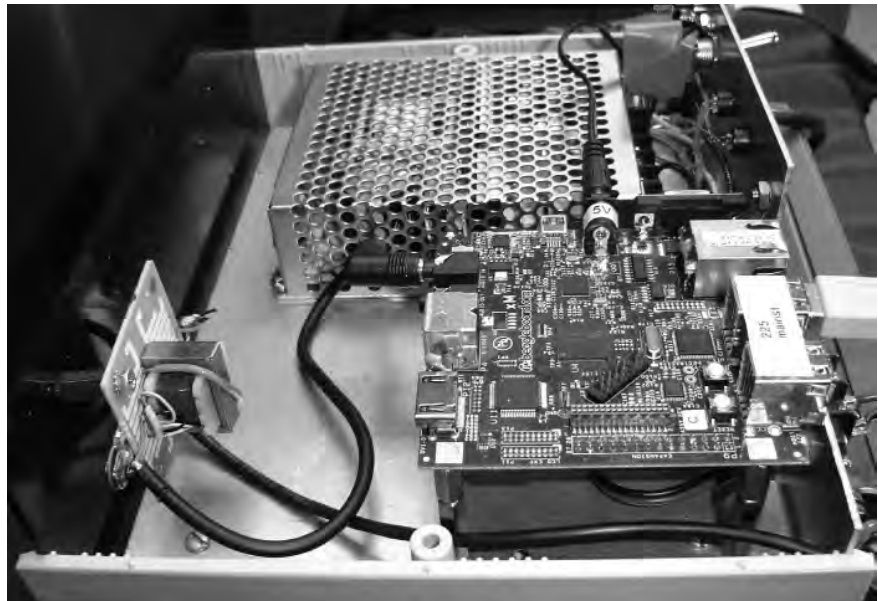
Figure 3 — This is an internal view of the remote control box. The BeagleBoard XM is in the lower right corner of the photo.
