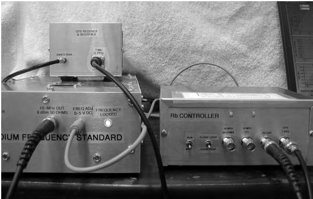
Figure 11 — Here is a view of the complete Rubidium oscillator frequency control system.
