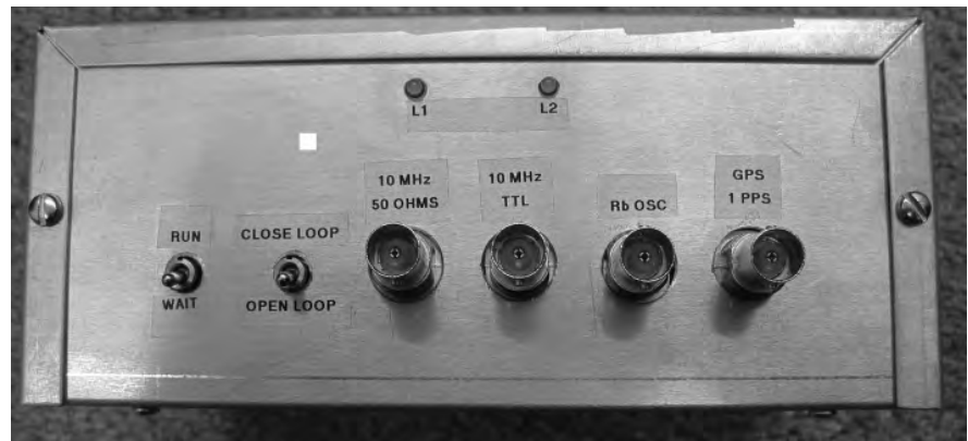
Figure 9 — Here is a photograph showing the front panel of the Rubidium-GPS frequency controller.
