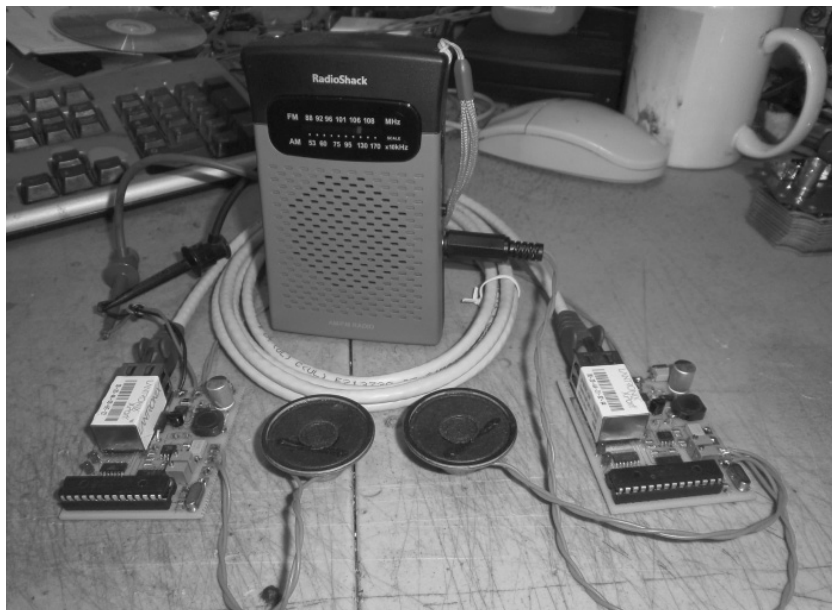
The author's test-bench setup for testing a pair of the VoIP boards.
